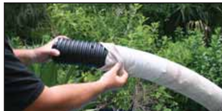
Fig. 8. 4" corrugated pipe used in the 55-gallon drum to contain coffee grounds
